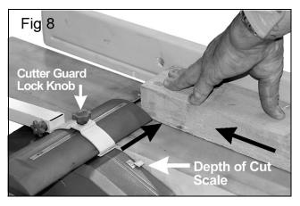
covering any exposed cutter. Ensure the guard is as low as possible and the cutter guard lock knob is tightened.
