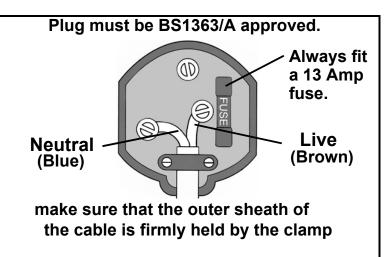
We recommend that this machine is connected to the mains supply via a Residual Current Device (RCD).
