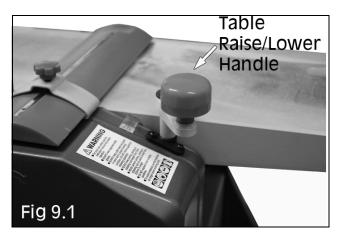
4. Withdraw the workpiece, then wind the table upwards - turn clockwise, using the Raise/Lower table knob, to the appropriate cutting depth (use the adjustment scale if needed), noting that one turn is equivalent to 3mm. **DO NOT** exceed 2mm depth of cut as this could cause kickback, and/or damage to the components or overheating of the motor.
