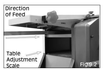
**NOTE:** It is advisable when working with rough or warped wood to make very small depths of cut to begin with - 1mm should be sufficient.
